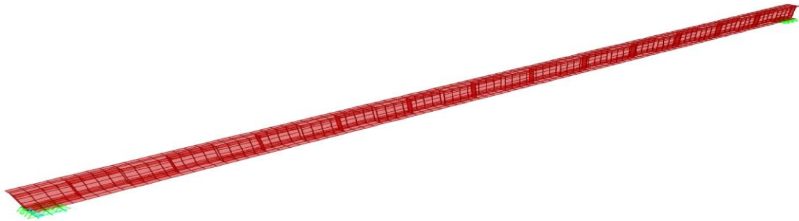
Fig. 2: 3D MODEL OF PLATE GIRDER WITH RECTANGULAR WEB
