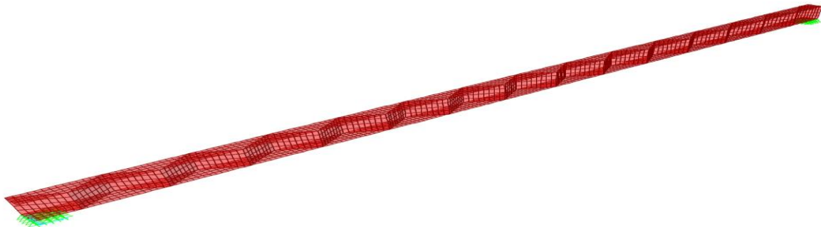
Fig. 3: 3D MODEL OF PLATE GIRDER WITH TRIANGULAR WEB
